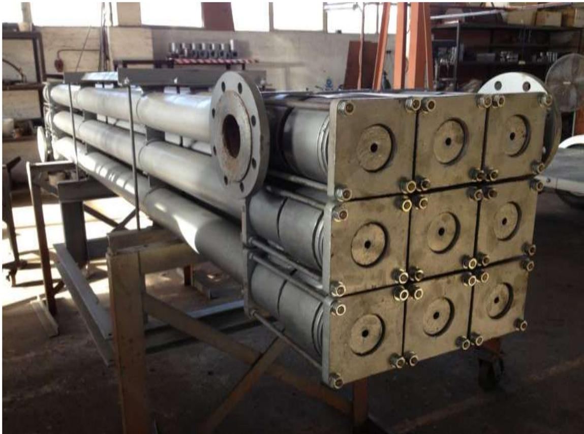
Figure 3: Mod-U-Flow Heat Exchanger (Picture: Amanda Botes)
